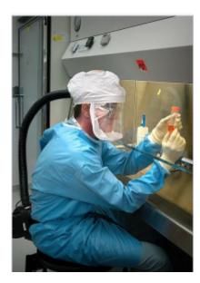
is a type of personal protective equipment used to safeguard workers against contaminated air. PAPRs consist of a respirator in the form of a hood, or full-face mask, which takes ambient air that is contaminated with one or more type of pollutant or pathogen, actively removes (filters) a sufficient proportion of these hazards, and then delivers the clean air to the user's face and/or mouth. PAPRs are sometimes called positive-pressure masks, blower units, or just blowers.
